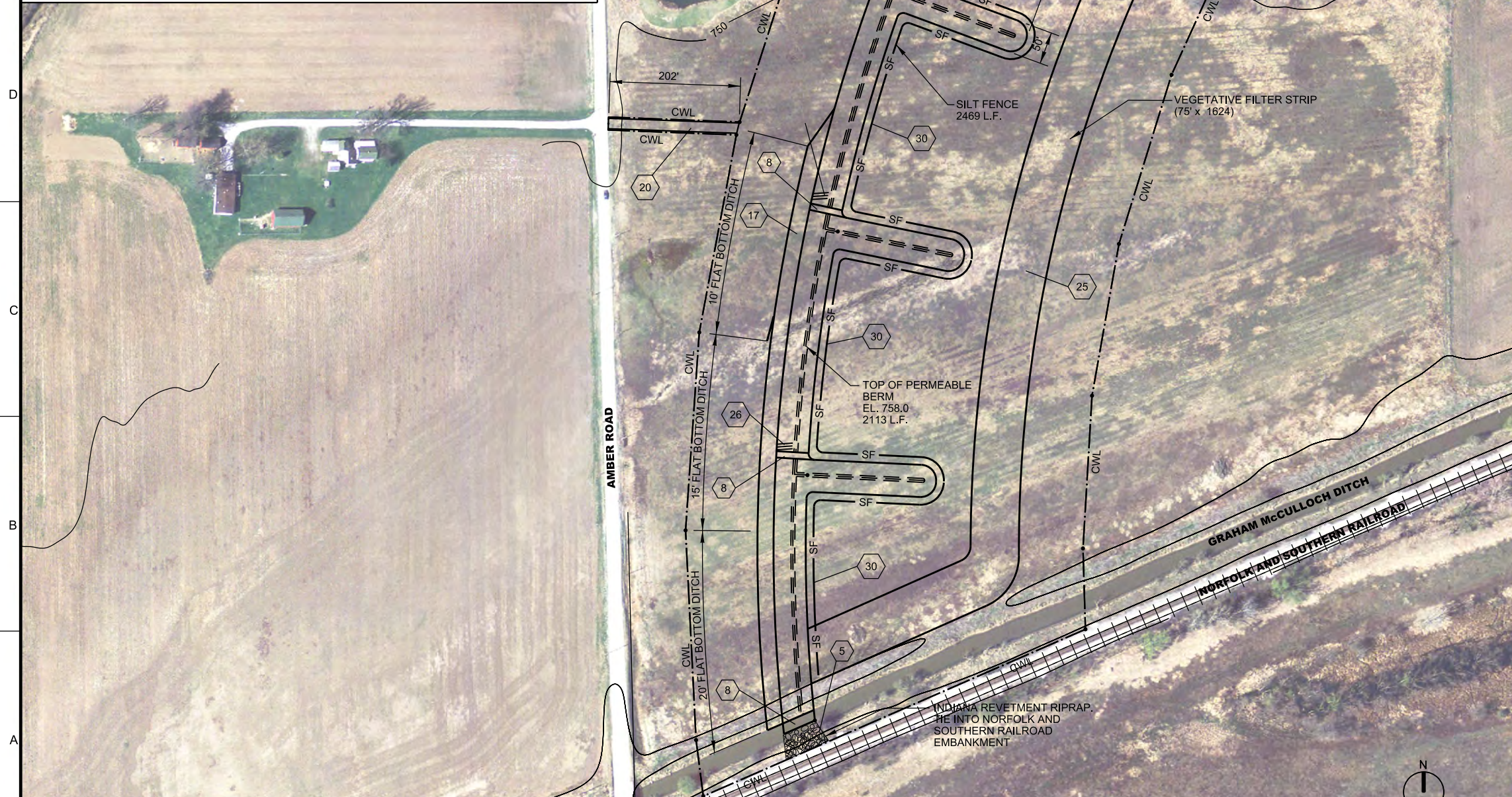
A1 ALTERNATIVE D CONSTRUCT PERMEABLE BERM WITH TELEMETERED SLUICE GATES ENLARGED SITE PLAN
