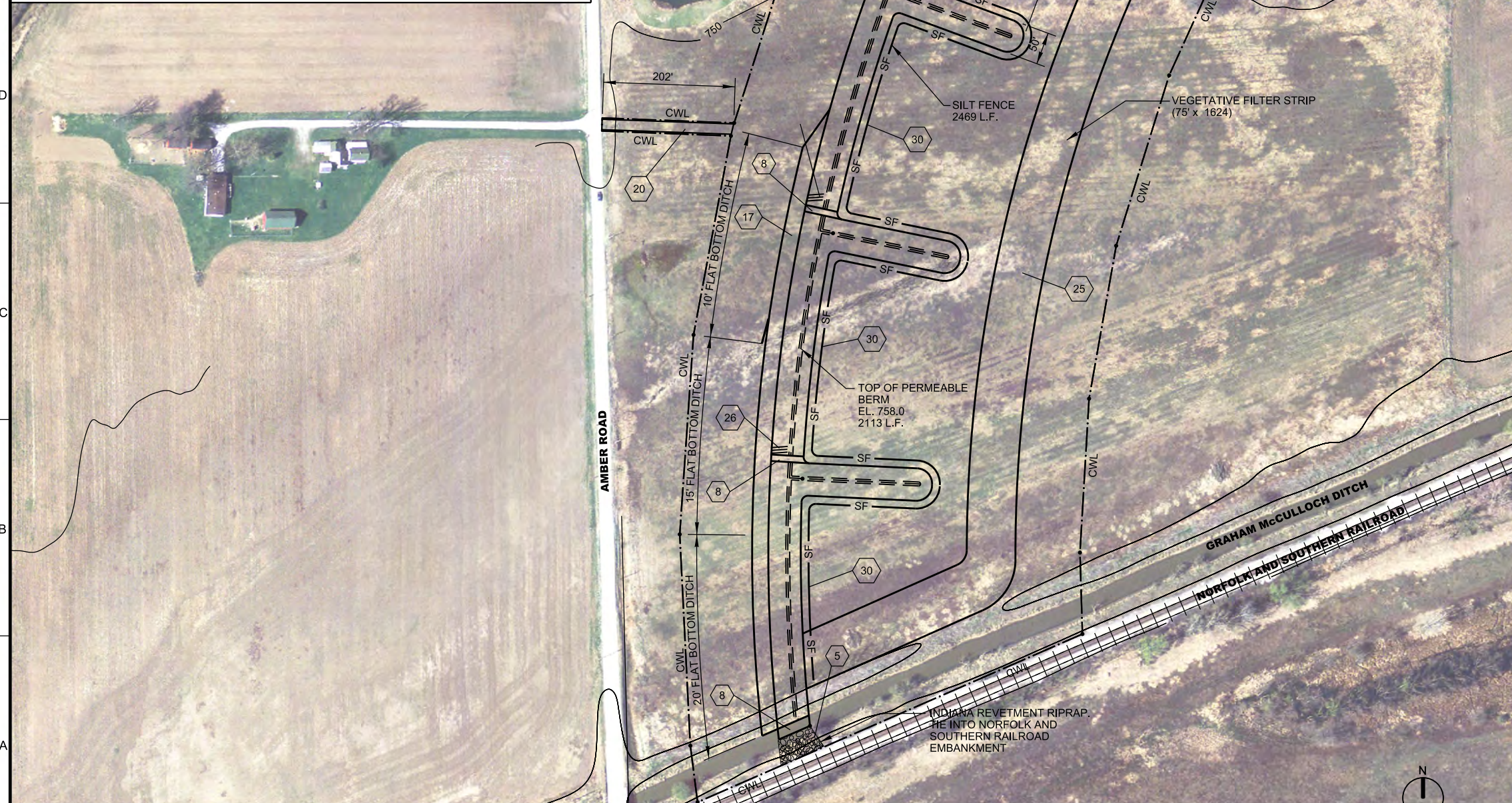
A1 ALTERNATIVE D CONSTRUCT PERMEABLE BERM WITH TELEMETERED SLUICE GATES ENLARGED SITE PLAN 1"=100'
