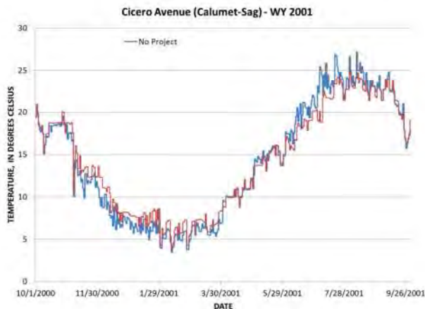
Figure K.8. (cont.) Comparison of Temperatures in the Chicago Area Waterways System for “No Project” and “Lakefront Separation” Alternatives for Future Conditions for Water Year 2001.
