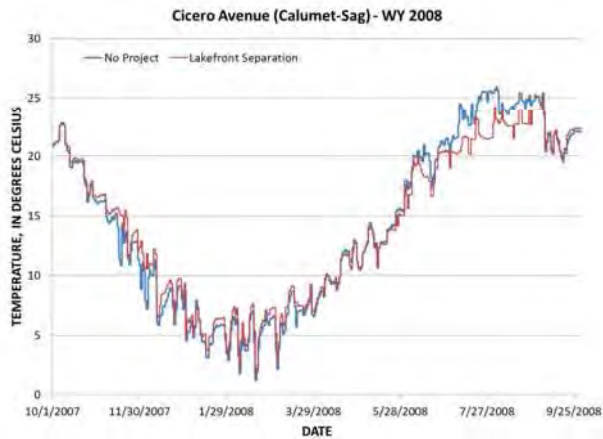
Figure K.12. (cont.) Comparison of Temperatures in the Chicago Area Waterways System for “No Project” and “Lakefront Separation” Alternatives for Future Conditions for Water Year 2008.
