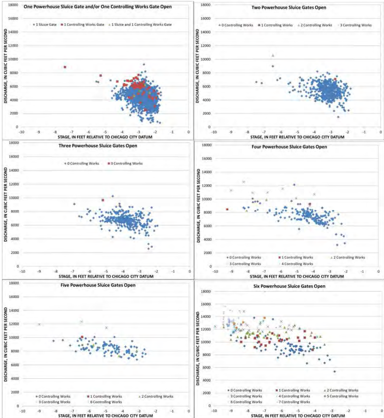
Figure 5.23. Relation between flow at Romeoville or Lemont and stage at the Lockport Controlling Works for the cases of one generator on at the Lockport Powerhouse and various numbers of powerhouse sluice gates and/or controlling works gates open.
