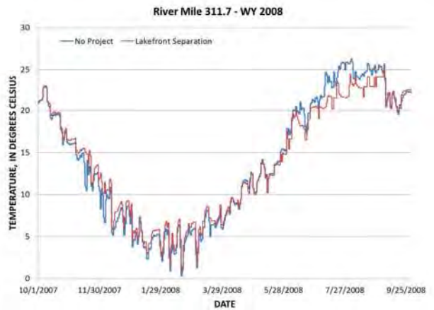
Figure K.12. (cont.) Comparison of Temperatures in the Chicago Area Waterways System for “No Project” and “Lakefront Separation” Alternatives for Future Conditions for Water Year 2008.
