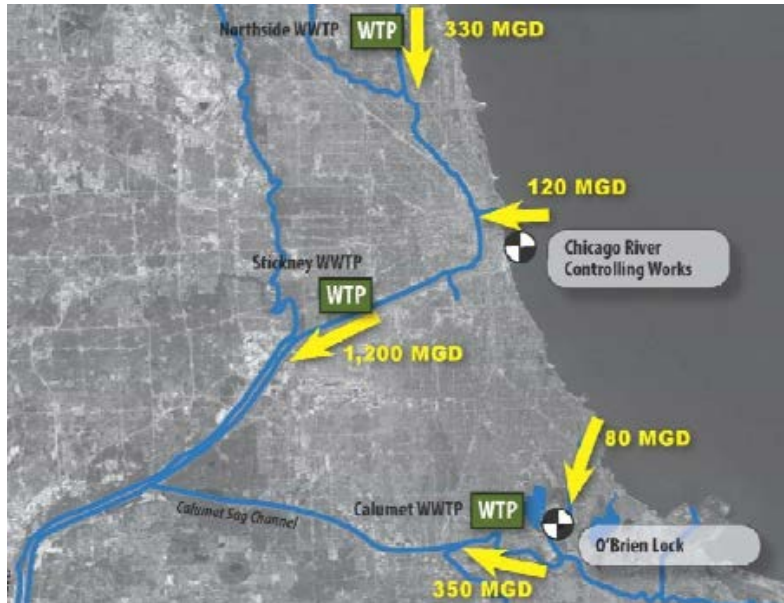
Figure 9. Waste Water Treatment Plants
