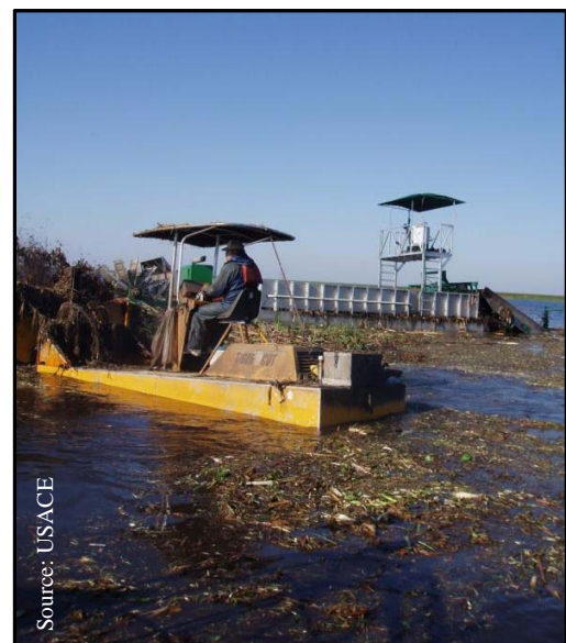
Tiger cutter barge and mechanical harvester working in conjunction to control aquatic vegetation in Monkey Box Run Lake Okeechobee, FL
