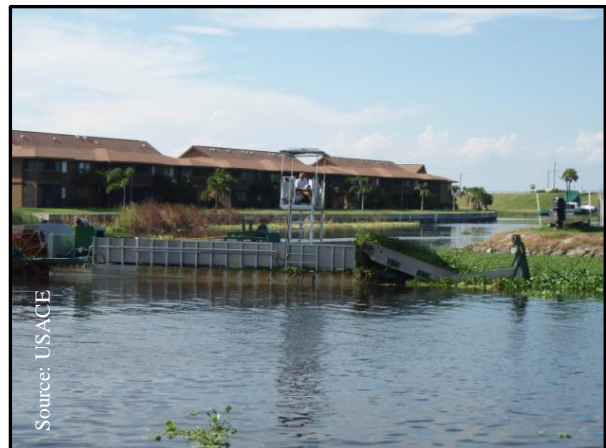
Mechanical harvester removing floating and emergent vegetation from a USACE boat basin in Clewiston, FL
