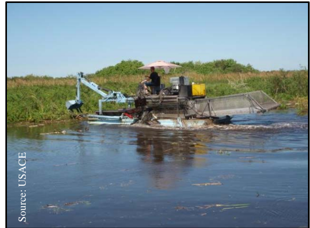
Mechanical harvester removing tussock material from Lake Hicpochee, FL
